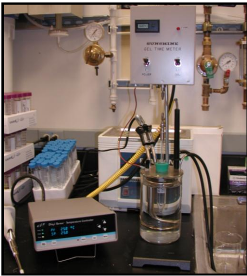
Figure 1: Sunshine Gel Time Meter ( http://www.davis.com )
