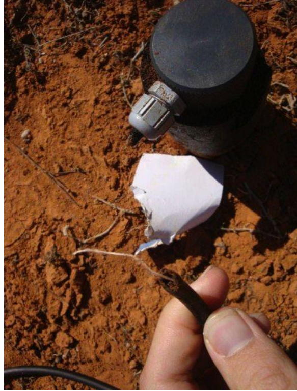
Figure 7: Data cable chewed off at its junction with the probe.
