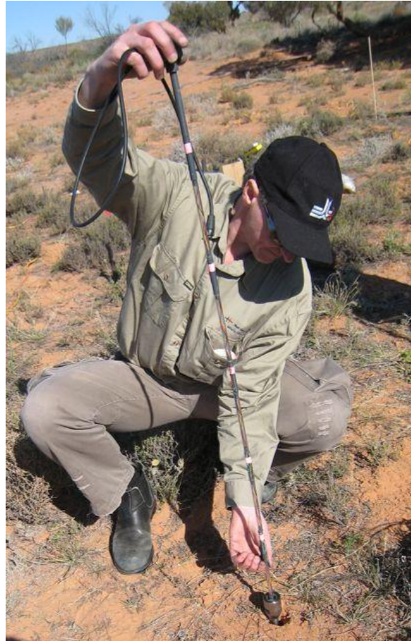
Figure 3: The author inserting a string of thermistors into one of the probe casings fully inserted in the ground.
