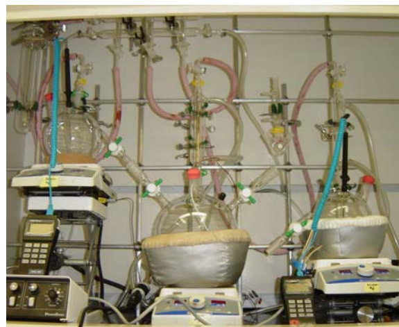
Figure 4. Photograph of high-reaction-volume synthesis set-up for up-scaled quantum dot production.
