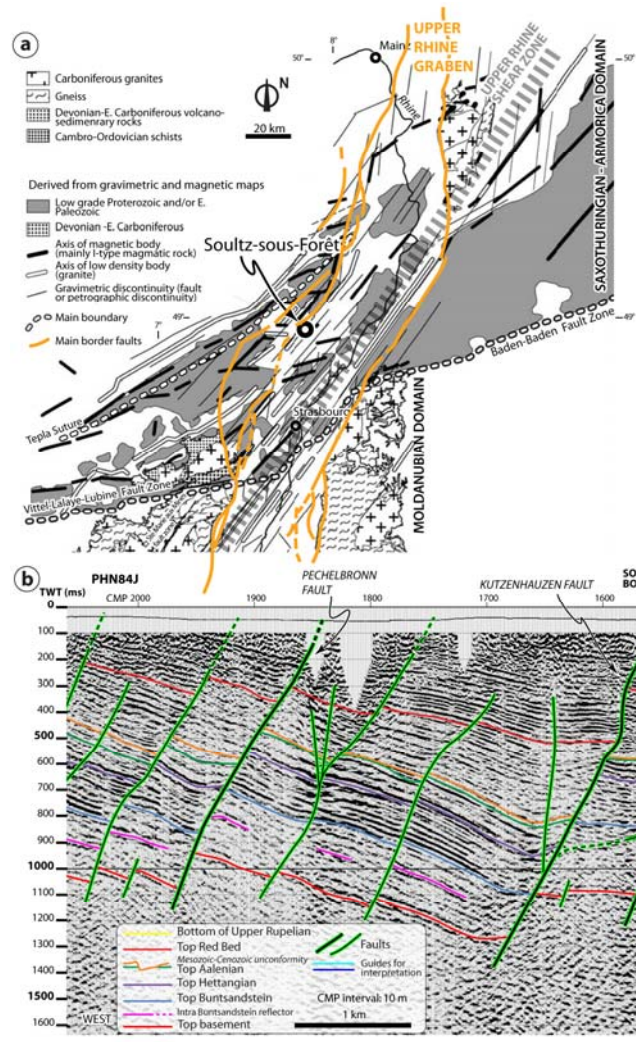
Figure 1: a) Position map of the Soultz-sous-Forêts EGS within the Upper Rhine Graben, illustrating variscan units and structures (modified after Édel and Schulmann (2009) and Édel et al. (2007)). b) E-W oriented reflection seismic profile, allowing to delineate much more structures in the sedimentary cover than in the crystalline basement. The arrow at the bottom of the profile indicates the position of a major fault zone indentified by other methods in the basement; the expression of this structure in reflection seismic is only a discreet flower-like structure in the sediments.
