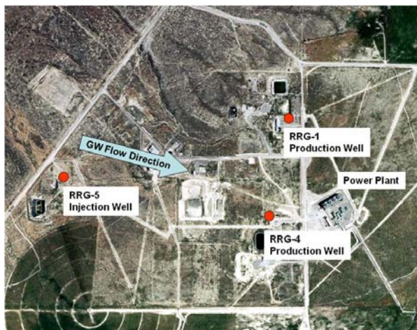
Figure 4: Aerial view of the central portion of the Raft River geothermal site indicating the location of the tracer injection well and the two closest production wells.
