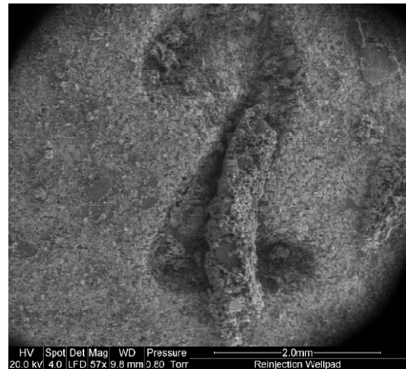
Figure 4: Low magnification of the 2 \mu\text{m} stainless steel filter from injection wellhead brine.
