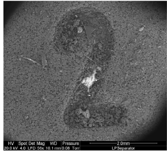
Figure 3: Low magnification of the 2 \mu\text{m} stainless steel filter from LP brine.
