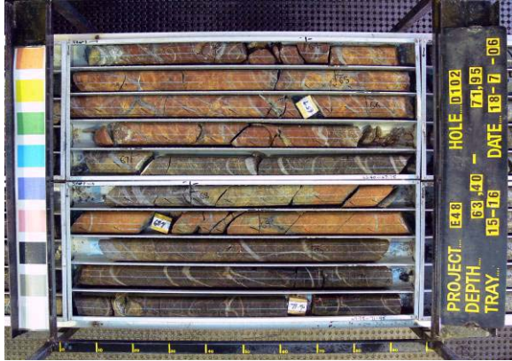
Figure 3: Core from E48D102. The reddish core is porphyry and the grey core is volcaniclastic.
