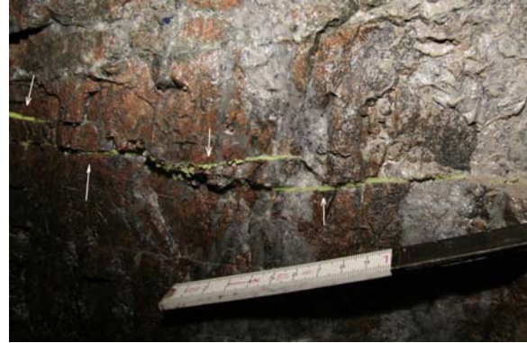
Figure 10: Fracture 8 on the south side of ED4, a few meters to the west of the structure shown in Figure xx7. A sequence of echelon fractures formed at this location.
