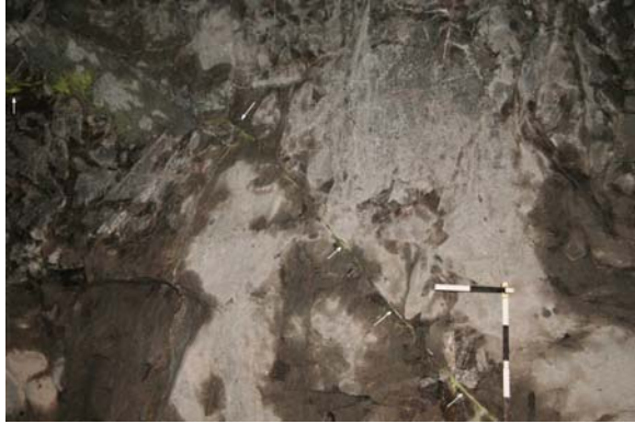
Figure 8: Offset 1 (see Figure 7) in fracture 8, on the south side of ED4. The scale is 100 mm for each black and white segment.
