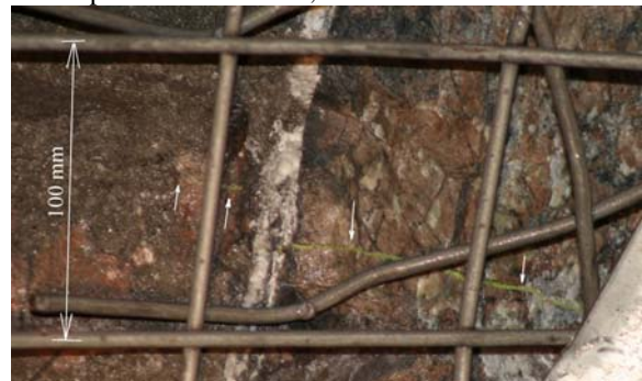
Figure 11: Fracture 8 on the south side of ED4. A small offset is shown in the path of the fracture as it crosses a vein.
