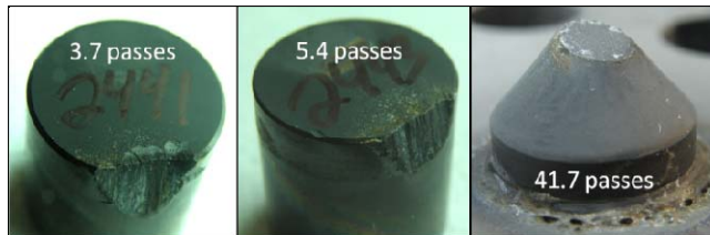
Figure 13: Non-leached, deep leached and stinger cutters after burn out during VTL testing.
