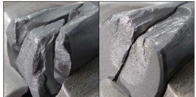
Figure 5 Results of initial VTL testing on low grade PDC shear cutters. Test included 50 passes, 0.050" depth of cut, 0.300" in-feed rate and 25 RPM.
