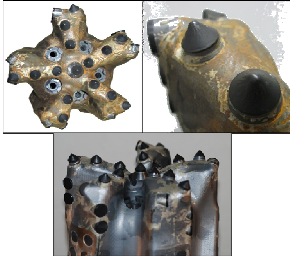
Figure 15. Stinger bit and blade detail after testing at Terra Tek geomechanics laboratory.
