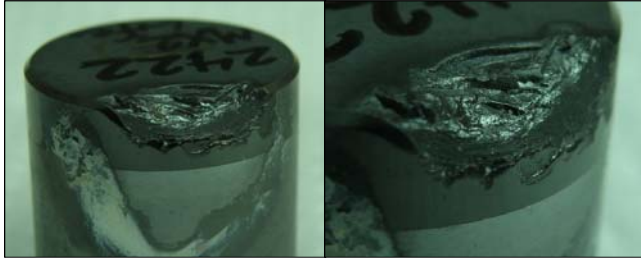
Figure 9: Shear PDC cutter following 75 passes on the VTL, 62,635 linear feet traveled.
