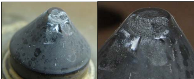
Figure 10: Stinger PDC cutter following 140 passes on the VTL.
