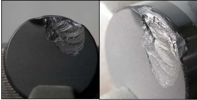
Figure 6: Results of initial VTL testing on premium (surface-leached) PDC shear cutter.
