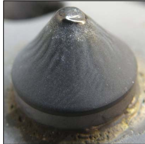
Figure 14. Stinger cutter at 25 passes during VTL hot testing.
