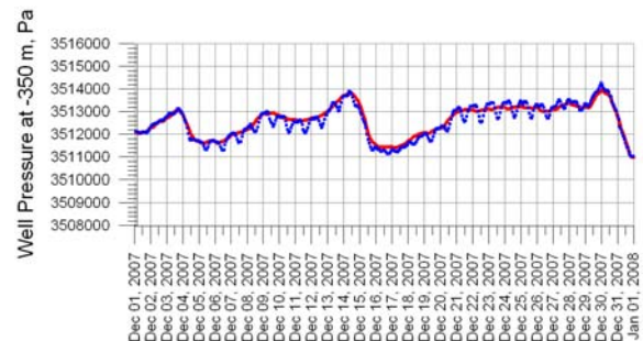
Figure 7: Match of short-term inverse modeling data: modeled well pressure (red lines), observational data (blue dots).
