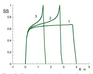
Figure 3. Non-stationary regime of salt precipitation after 100 years for  $P_0 =$  $1.87 \cdot 10^7$  Pa (line 1). Reservoir sealing after 66 years for  $P_0 = 1.885 \cdot 10^7$  Pa (line 2). after 20 years for  $P_0 = 1.89 \cdot 10^7$  Pa (line 3).
