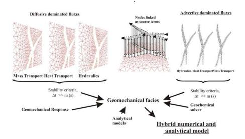
Figure 8 Conceptual illustration of a multiple mesh hybrid numerical analytical mdoel for HTMC coupling based on the geomechanical facies approach
