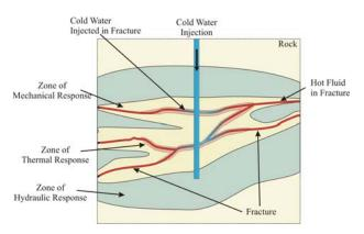
Figure 1 Different processes operate at different scales, example for hydraulic, mechanical and thermal processes.
