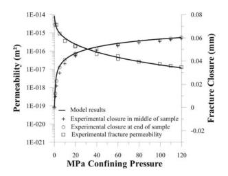
Figure 5 Functional approximation of permeability with stress.
