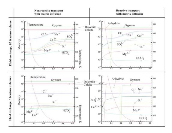
Figure 9 Comparison between non reactive and reactive transport modeling of the mixing of hot geothermal fluid and seawater in carbonate and gypsiferous fractured rock.
