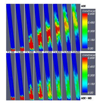
Figure 7 Realistic fracture profile, transport of a tracer with (lower) and without (upper) the influence of matrix diffusion.
