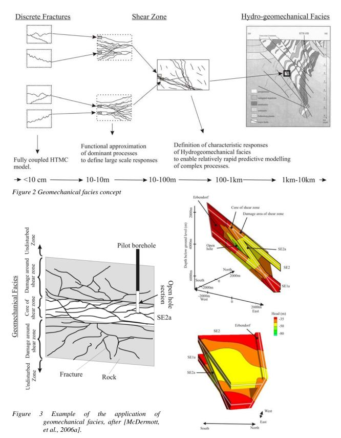
Figure 4 Three dimensional combination of the geomechanical facies at the KTB site, [McDermott, et al., 2006a].
