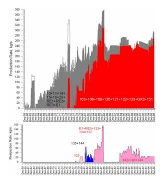
Figure. 2. Extraction (above) and reinjection (below) rates during exploitation period 1960-2006 year. Old North Site production wells – grey, cold water reinjection – blue, 100-120°C reinjection –pink color.
