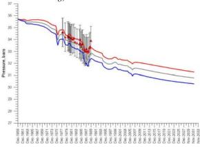
Figure. 5. FOSM error propagation analysis of the Pauzhetsky model applied to well #124 pressure forecast for 1960-2032 year. Lines – 95% confidence interval for the model. Triangles – observation data. Bars – 95% confidence interval for observations (standard deviation of pressure measurements assumed as  $\sigma$ =0.3 bars).
