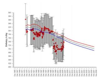
Figure. 4. FOSM error propagation analysis of the Pauzhetsky model applied to well #106 enthalpy forecast for 1960-2032 year. Lines – 95% confidence interval for the model. Triangles – observation data. Bars – 95% confidence interval for observations (standard deviation of enthalpy measurements assumed as  $\sigma$ =20 kJ/kg).
