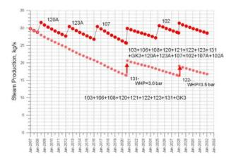
Figure. 7. Modeling forecast for steam rate at separation pressures of wells 103, 106, 108, 120, 121, 122, 123, 131, GK3, 120A, 123A, 107A, 102A for time period of exploitation 2007-2032 year.
