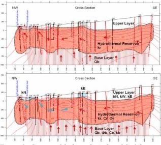
Figure. 1. Conceptual hydrogeological model of the Pauzhetsky geothermal field and parameterization of corresponding numerical model: natural state (above) and exploitation (below).
