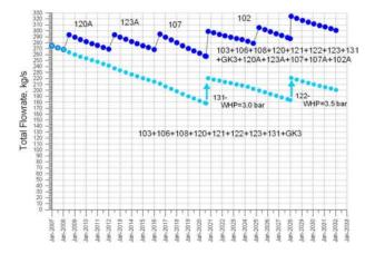
*Figure.6. Modeling forecast for total flowrate of wells 103, 106, 108, 120, 121, 122, 123, 131, GK3, 120A, 123A, 107A, 102A for time period of exploitation 2007-2032 year.*
