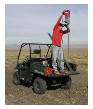
Figure 2. Hollow steel temperature probe being driven into ground with electric demolition hammer.
