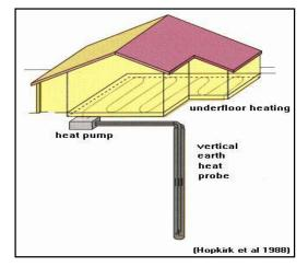
Fig. 2. Borehole- Vertical Heat Exchanger-Geothermal Heat Pump System for space heating and cooling scheme.
