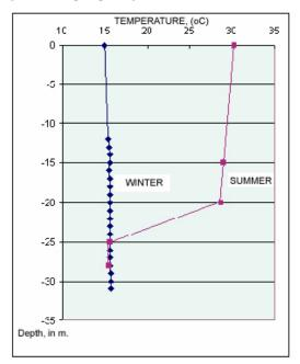
Fig. 4. Thermolog of the Rinasi borehole
