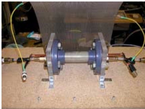
Figure 3: Core sample testing device with Berea sandstone. Core is 127 mm long and 25 mm diameter. Copper screws are electrodes.
