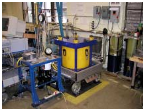
Figure 1: Triaxial testing device including (from left to right) data acquisition digitizer, injection pump, true-triaxial cell, and air/hydraulic intensifiers. Boiler is in background behind injector.
