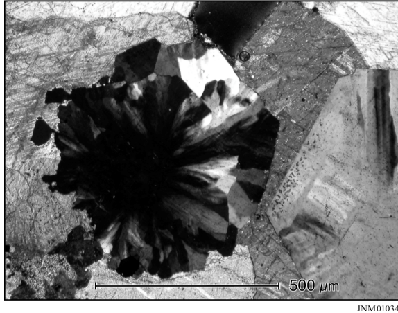
Fig. 4. Quartz with strongly corroded crystal faces from 1214.3 m in K-33. The complex extinction pattern suggests deposition from boiling fluids. The quartz is surrounded by later calcite.
