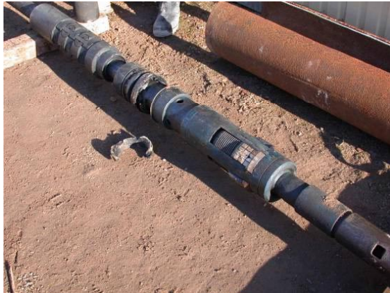
Figure 8: Mechanical packer used successfully in the sandstone stimulation experiments.
