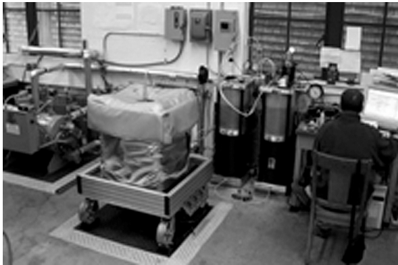
Figure 3 Overview of the testing device. From the left of the picture: boiler, pressure cell with insulation jacket, pressure intensifiers, computer control station (Talesnick in command).
