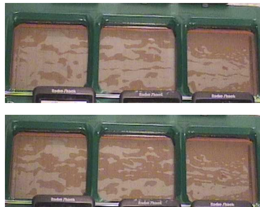
Figure 3.3 Examples of gas flow path increase in width as gas flow rate increases and water breaking up this flow path.
