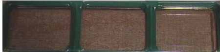
Figure 3.17 Picture of wave-like fronts seen in high gas-water ratio at imbibition experiment.
