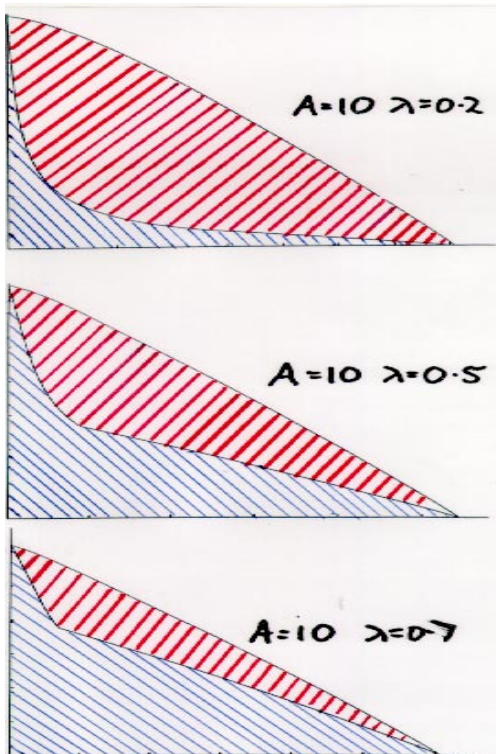
Figure 3 Structure of reaction front produced in strong dissolution reaction. In these calculations, the reaction zone extends all the way to the front of the region occupied by injected liquid. Numbers on the curves represent different values of \lambda . Here K=10 .
