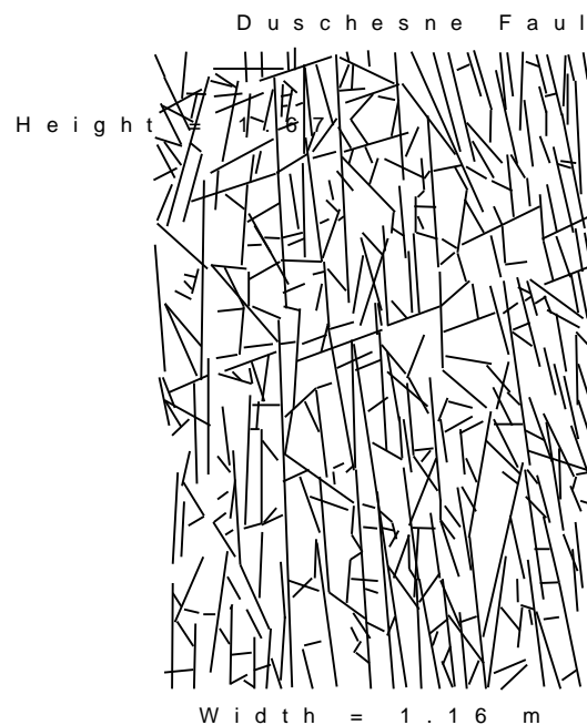
Figure 1b: Bedding surface fracture pattern.
