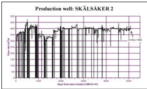
Figure 4. The flow rate recorded in the production well Skälsåker 2.
