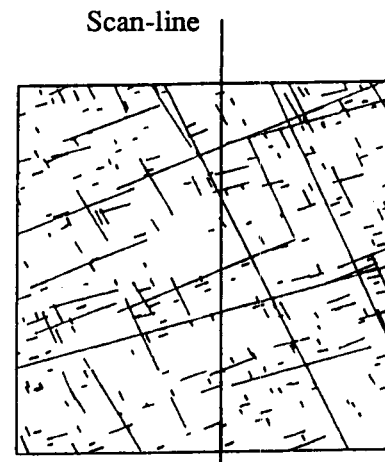
Fig. 7. Fracture network simulated by means of fractal relation
