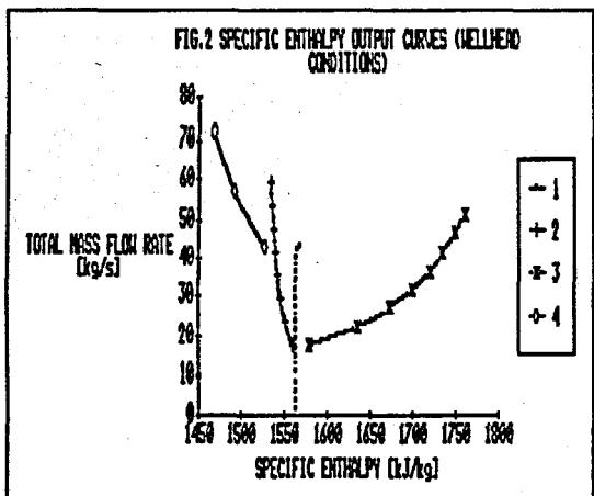
Curves 1 in both figures represent the production output curves assuming a single feed zone located in a point at 1800m depth where the formation conductivity ( $kh_1$ ) is  $5 \text{ E-13 m}^3$ , and the thermodynamic state of the fluid under static conditions is defined by:  $P_{y1} = 17.5 \text{ MPa}$ ; and  $h_{y1} = 1580.3 \text{ kJ/kg}$ , noticing that only pure-water is considered.
