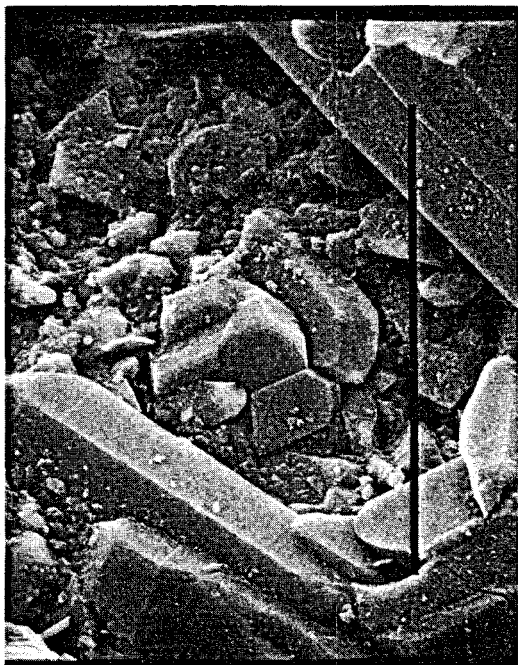
Figure 5. Authigenic albite (center) and euhedral quartz crystals in fracture-dominated flow zone from East Brawley. Bar = 1 micron.
