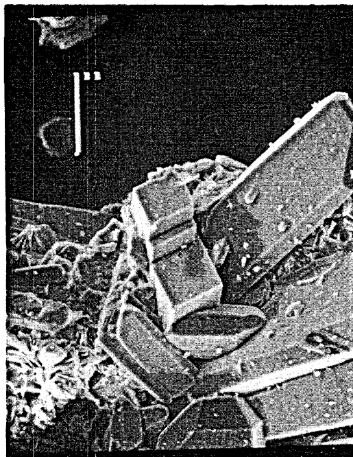
Figure 6. Euhedral quartz crystals, calcite rhombs, and leafy aggregates of chlorite (lower left) indicate equilibrium growth in assemblages lining fractures. Bar = 100 microns.
