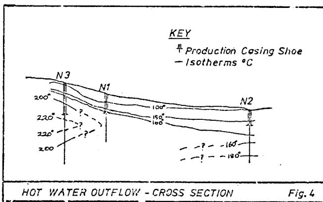
The Okoy geothermal field cross sections (Smith, 1980 b) suggested wells N3, N1 and N2 are in an outflow from the Upper Okoy reservoir with OK3 in the outflow edge.
