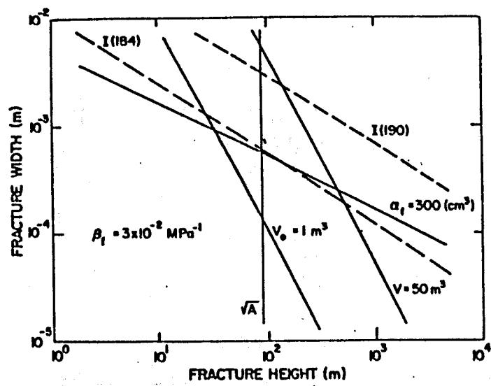
FIG. 5: APPROXIMATE FRACTURE DIMENSIONS
