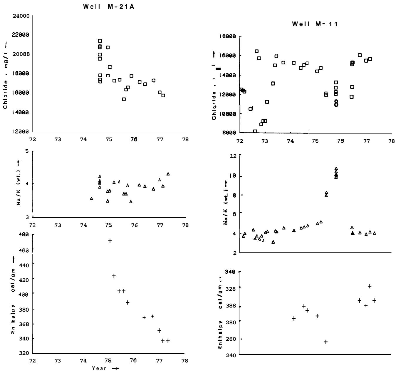
**Figure 2.** Chloride contents after flashing and the sodium to potassium ratio of brine and enthalpy of the total discharge of well M-21A from 1975 to mid-1977 and well M-11 from 1972 to mid-1977.. Data from Manon et al. (1977). Units are mg/kg, weight ratio and Kcal/kg.
