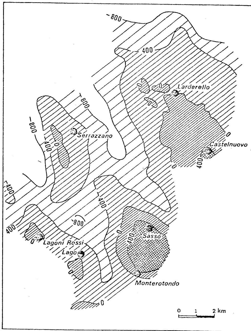
Figure 2 : Altitude of potential reservoir top in Larderello field ( m a.s.l.)
