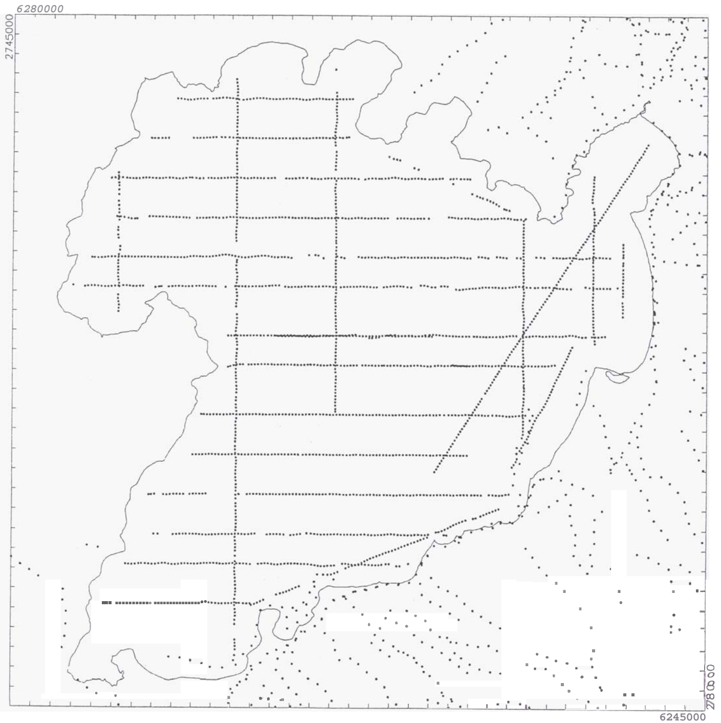
Figure 3. The map shows the positions of the resistivity measurements used to compile the contour map shown in Figure 4. These measurements are made up from three different data sets: measurements made on land using Schlumberger and Wenner arrays, waterborne measurements using anchored Schlumberger arrays with the electrodes placed on the lake bottom and waterborne measurements using a towed equatorial dipole-dipole array.
