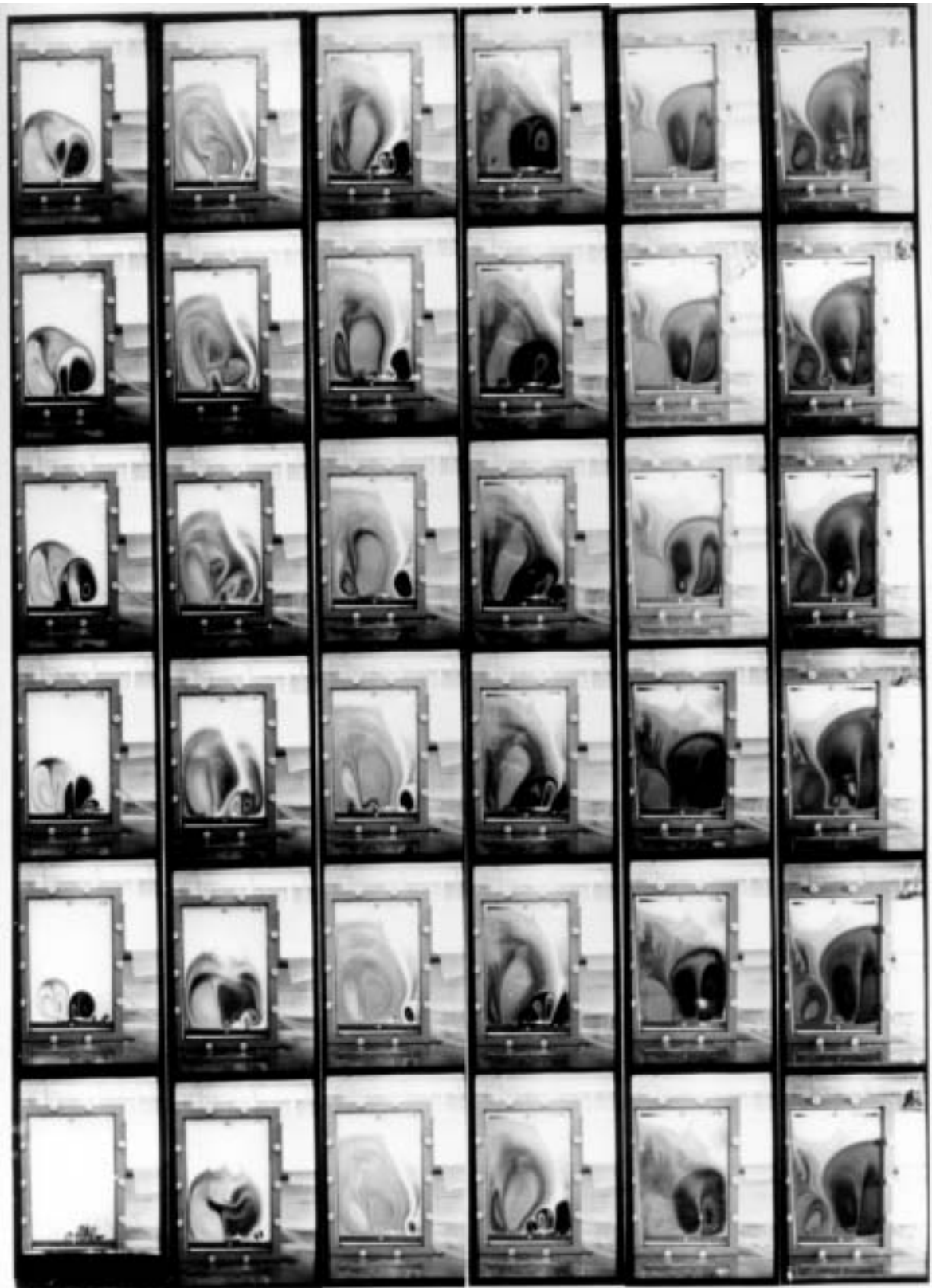
Figure 3.2: Experimental Solution for Rayleigh Number of 1600 - Fully Heated Boundary. Sequence recorded at 5 minute intervals.
